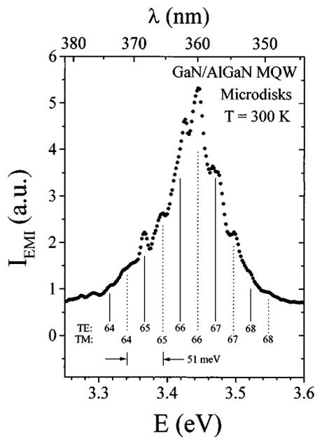
FIG. 2. Room-temperature PL spectrum from a single GaN/AlGaIn MQW microdisk showing radial ( $m=0$ ) optical resonance modes. Equally spaced lines show the approximate spacing of TE and TM modes (51 meV). The radial mode number and type (TE or TM) are also indicated.
